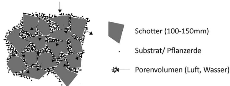
Abb. 55: Skeletterde (structural soil)
